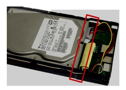
**Step 4** Secure the drive to the plate on the sides with the provided four screws.
